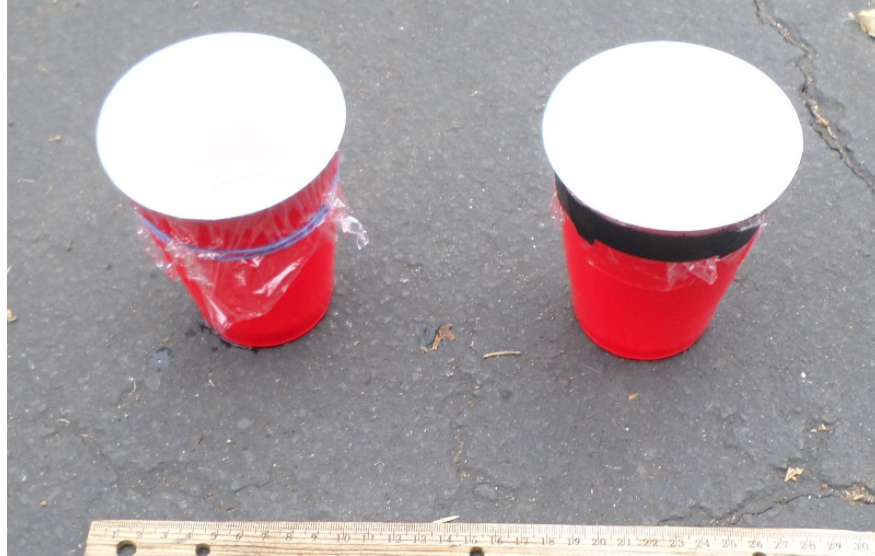
RANGER build photo #42: Potential venting area cups covered with plastic wrap. Note the two methods that can be used to secure the plastic wrap. The cup on the left uses rubber bands. The cup on the right uses tape.
