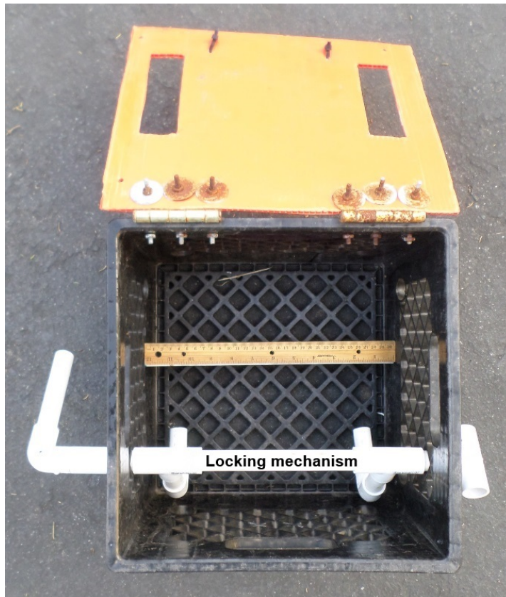
RANGER build photo #31: Locking mechanism inside the milk crate.
