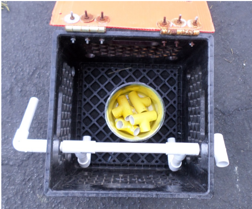
RANGER build photo #35: Cargo container open with grain cargo (yellow) inside.
