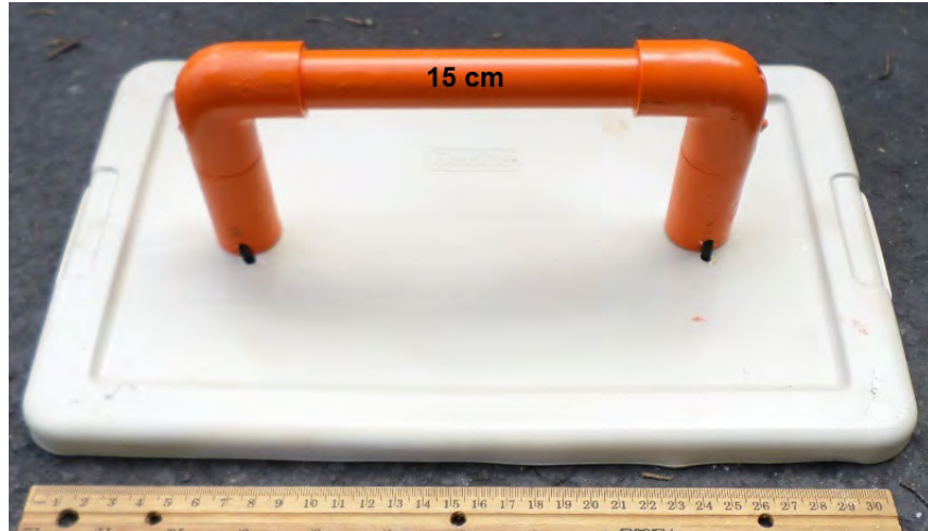
SCOUT build photo #1: The handle attached to the lid of cargo container.
