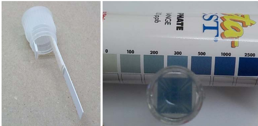
Left: Preparing the test strip in the cap of the sample bottle.
