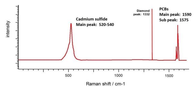
Raman spectrum of sediment contaminated with CdS (520-540 cm<sup>-1</sup>) and PCBs (1590 and 1575). Note the diamond peak (1332 cm<sup>-1</sup>).
