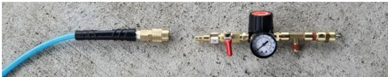
Connection to the MATE compressor.
