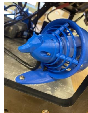
Figure 10: Front of the custom thruster guard featuring a wolf head.
