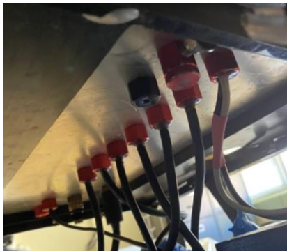
Figure 16: Wire Penetrators on Bottom of Electronics
