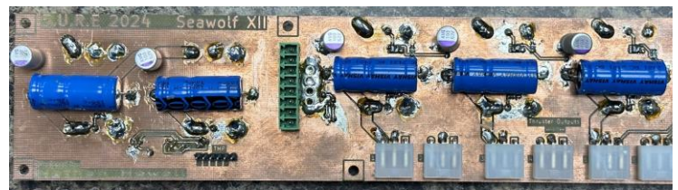
Figure 13: Top of Power Supply Board
