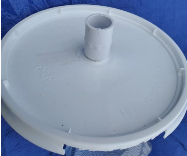
Left: The 3/4-inch female adapter attached. Right: Plastic cling wrap secured over the top of the 3/4-inch female adapter.
