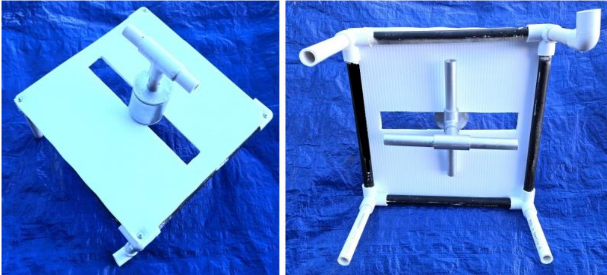
The sacrificial anode installed. Left: Top view. Right: Bottom view.
