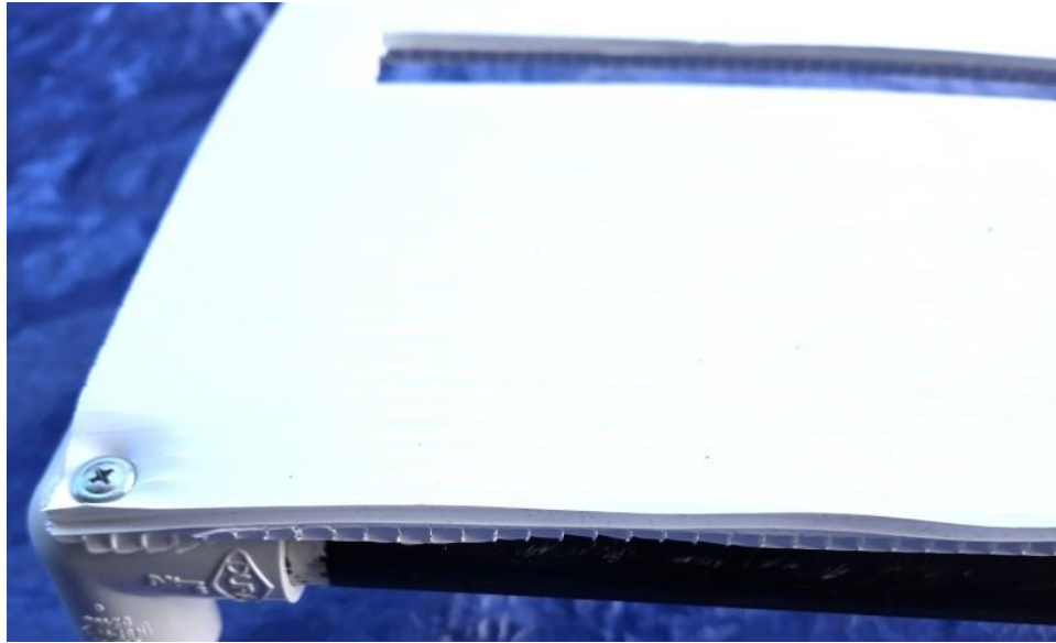
The double layer of corrugated plastic sheeting. The ribbing of the two sheets are offset to provide additional strength.
