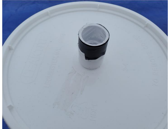
Left: The 3/4-inch female adapter attached. Right: Plastic cling wrap secured over the top of the 3/4-inch female adapter.
