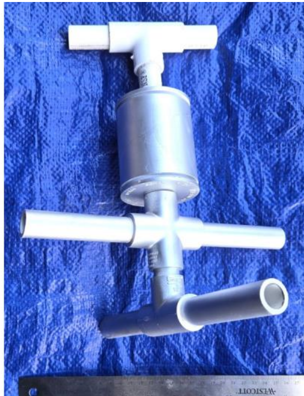
Both the old and the new sacrificial anode are constructed from 2-inch and \frac{1}{2} -inch PVC pipe. Left: The anode. Right: The anode painted silver.
