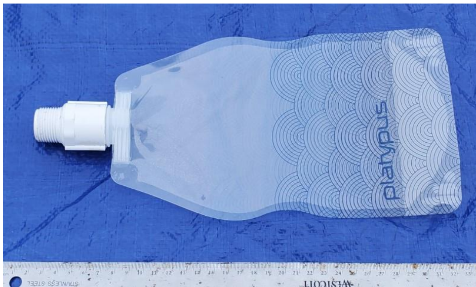
A 1 liter soft water bottle . Epoxy secures a ¾-inch male adapter to the mouth of the bottle.
