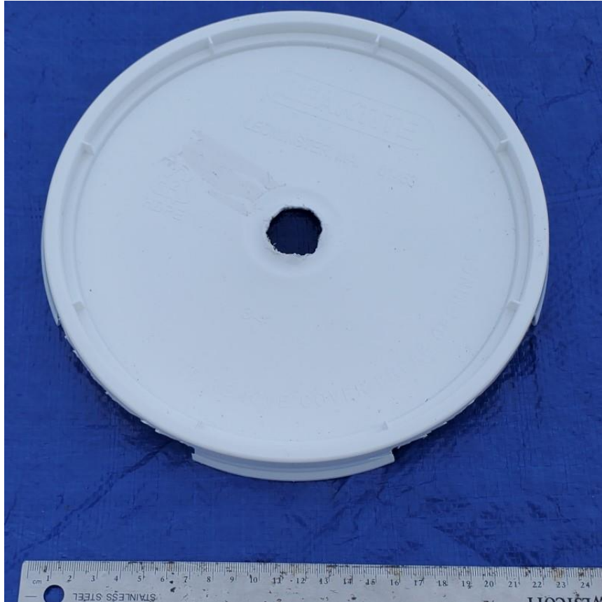
A 2-gallon bucket lid. The hole in the center is large enough for the threaded end of the \frac{3}{4} -inch male adapter to fit through.
