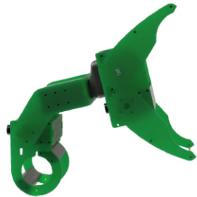
Figure 29.2 2-axis claw CAD
