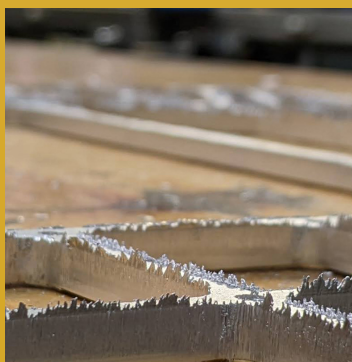
Fig. 4 - Pre-reamed frame with burrs attached
