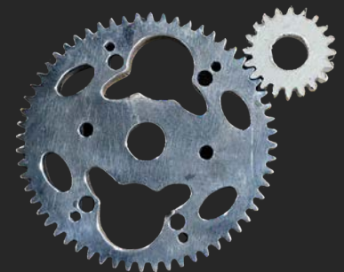
Proprietary gears used to rotate our gripper. they were outsourced to another dept. to be cut on a fiber-laser out of aluminum billet.
