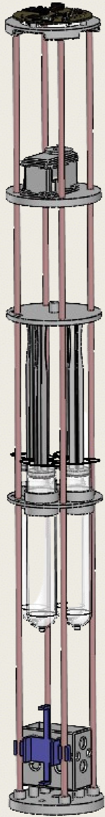
1. float's internal view
