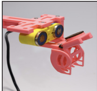
Figure 34. Photo of the BEM with the adapter and Sediment Sample Claw attachment
