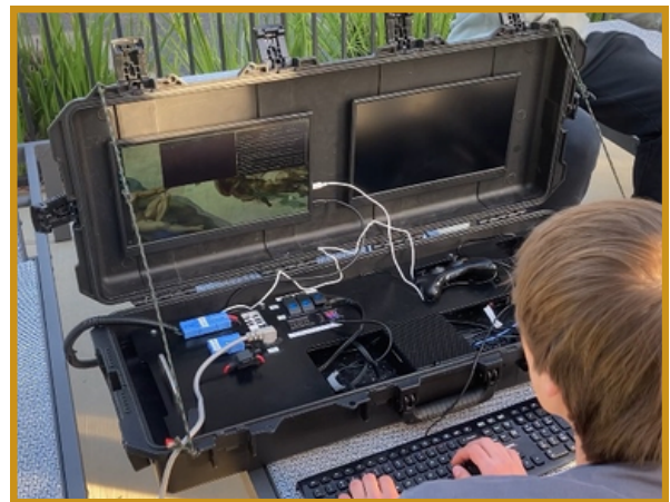
Figure 10: Control Station for ROV
