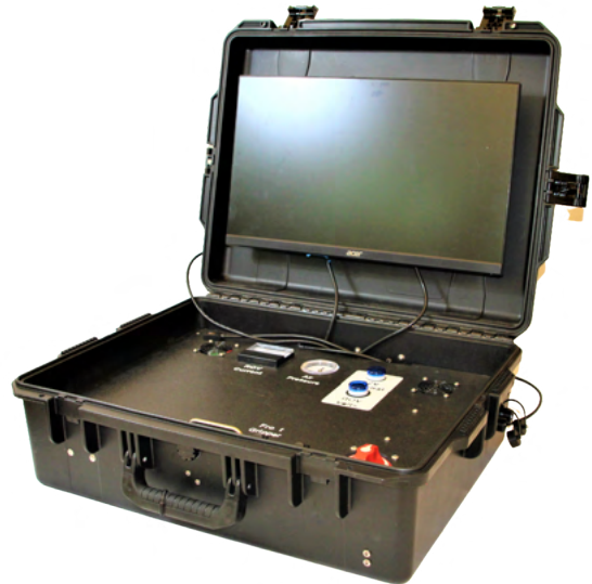
Figure 20. Topside Control Unit (TCU)
