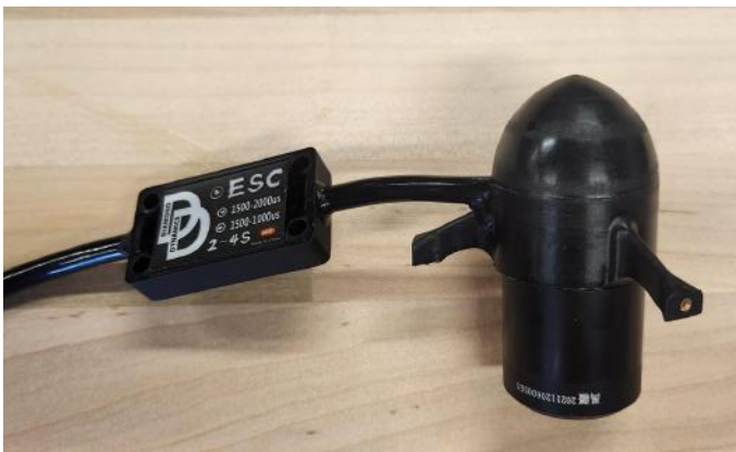
Figure 34: Repurposed 12V Diamond Dynamics Thruster
