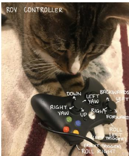
Figure 25: ROV Control Scheme
