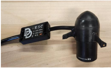
Figure 9: Spare Thruster Core Used for Claw Motor
