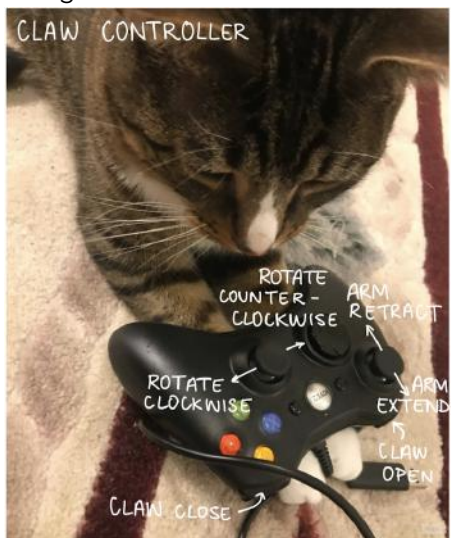
Figure 26: Claw Control Scheme
