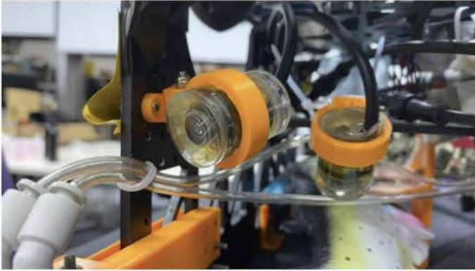
Fig.11 Analog cameras positioned on frame
