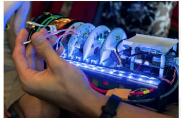
Fig.31 Backplane with Fail safe system and LED Display
