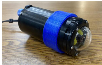
Photo of analog camera in enclosure. Credit: Gavin Bentley
