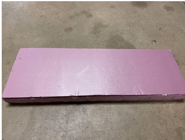
Figure 8: Foam Used For Additional Buoyancy
