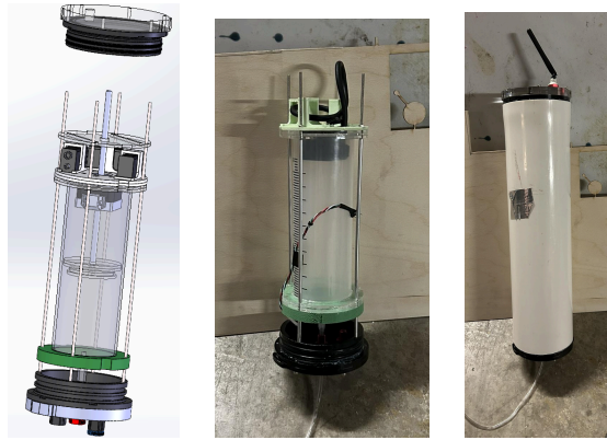
Figure 1: Float CAD without PVC Hull (left), Float internals (middle), and Float with PVC Hull (right)
