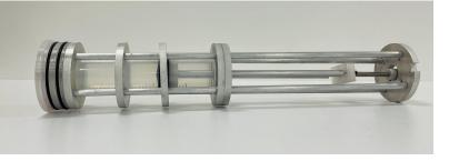
two plunger rods with a brass nut that is driven by a lead screw attached to our motor.
