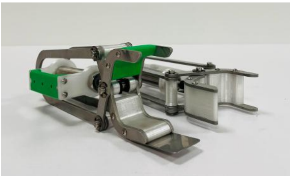
Fig. 6. Vertical (back) and Horizontal (front) Linkage Claw
