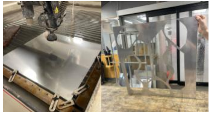
Fig. 2: Set-up and aftermath of Waterjetting
