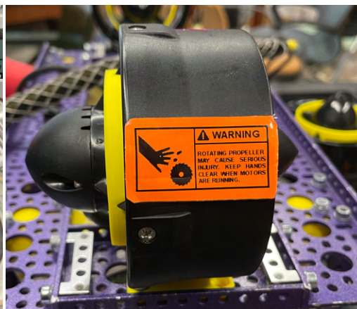
Figure 16B (above): Warning labels on thrusters follow ANSI Z535.3-2011 for safety symbols (ANSI, 2011).
