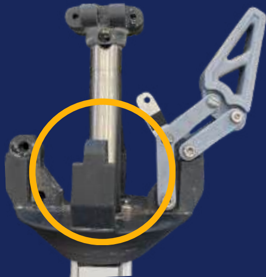
Fig. 43 Gripper linear actuator mechanism
