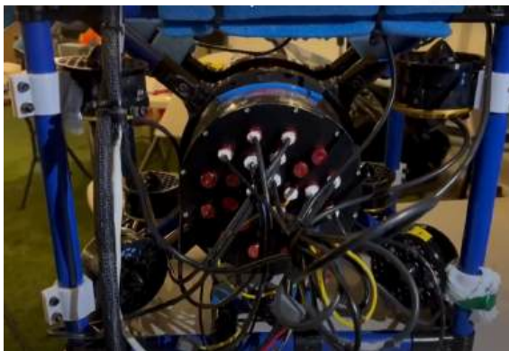
Fig. 8 Watertight enclosure and sealing
