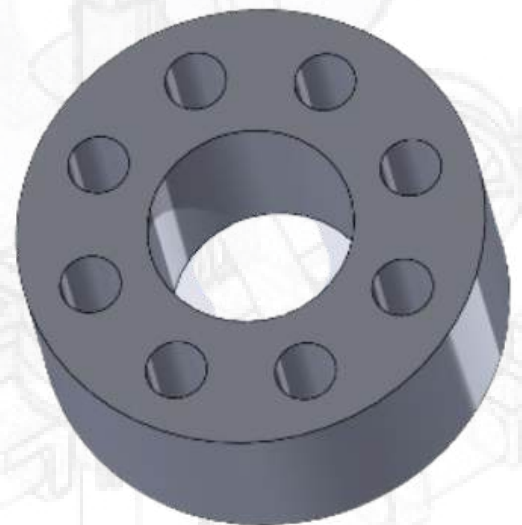
Fig. 18 CAD design of battery holder
