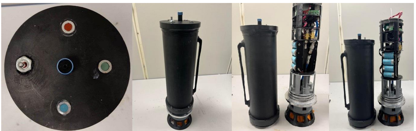
Figure 1: From the left is the top of the float with LED's, PRV, and power switch. Next is the float fully assembled. Third and fourth from the left is the float with the sleeve disassembled from the electronics.
