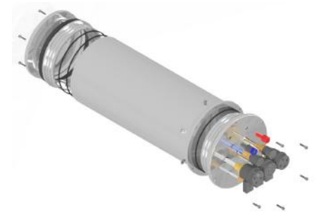
Figure 6: Exploded view of the electronics enclosure.
