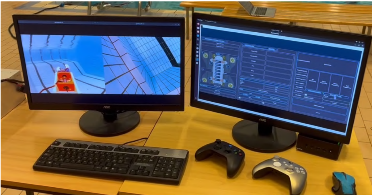
Figure 28: Topside system setup.
