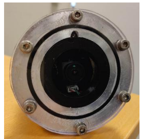
Figure 20: External camera house. Camera type: Waveshare OV2710. Maximum resolution: 1920x1080. Camera sensor: OV2710.
