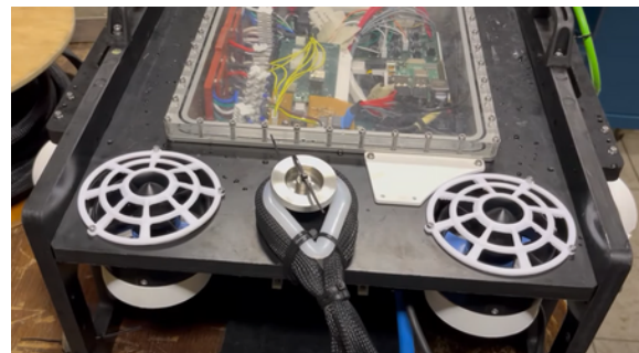
14 - Bottom side strain relief
