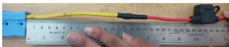
20A Littelfuse is within 30cm of the Anderson Connector
