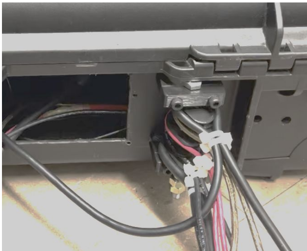
Figure 9: Control Station strain relief.
