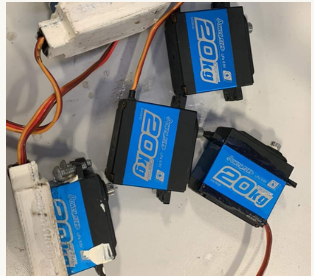
Fig. 22. Waterproofed servo motors
