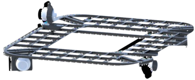
Fig. 23: ROV Frame and Camera positions (Front of ROV is bottom in this image)
