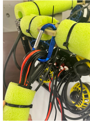
Figure 8: Tether strain relief before entry into watertight enclosure.
