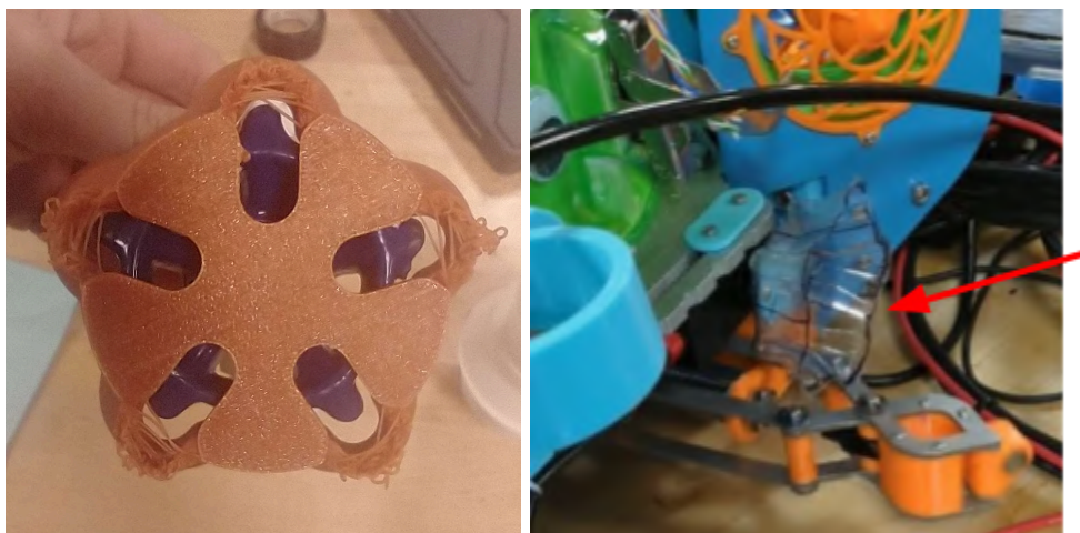
Fig. 16: Valve manipulator prototype (left) and final integration (right)
