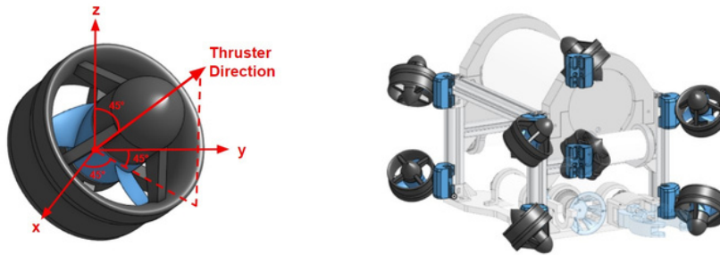
Figure 15: Diagram of the thruster direction (left) and thruster placement on Beaumont (right), Mark Johnson, 2024
