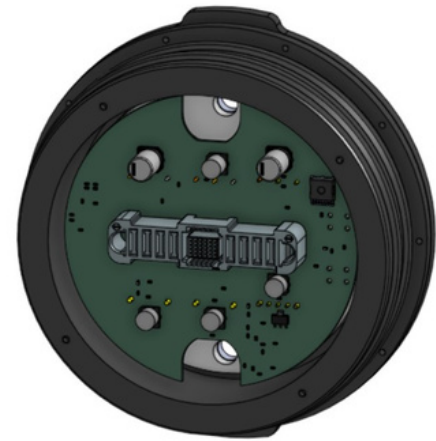
Figure 7: Power Conversion Board, Mark Johnson 2024
