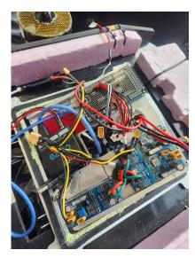
To control the ROV we use a controller attached to the jetson nano. The jetson nano interprets the direction it is supposed to go or other commands then it sends that down to the arduino. The ROV also sends camera feed back up to the jetson nano. This allows us to control the ROV and complete the tasks.
