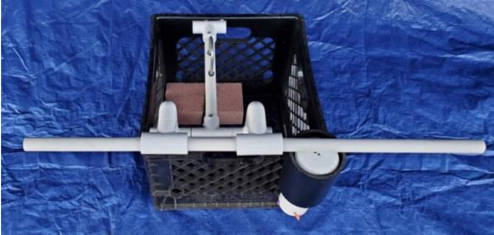
The multi-function node with the acoustic release pin holding the recovery float in place.
