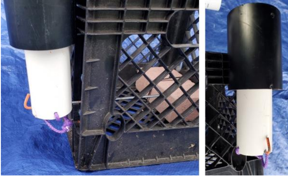
Left: The pin holding the recovery float. The recovery float rope is stored inside the float, above the pin. The pin passes through a loop in the rope, holding the rope in place until the pin is removed. Right: Two notches drilled into the bottom of the recovery float hold the pin in place.
