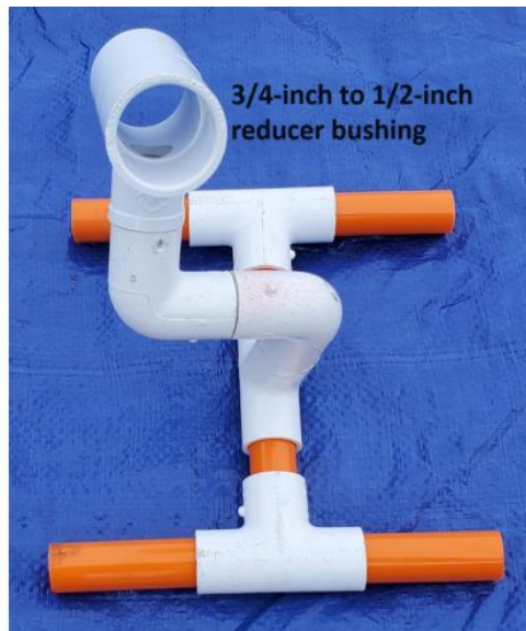
Left: Acoustic receiver front view constructed from 1/2-inch PVC pipe. Right: Acoustic receiver side view.
