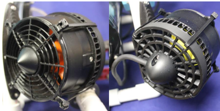
Front and back views of the ROV's thrusters. Photos by Rachel Smith.
