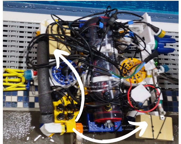
Figure 6. Spikes' buoyancy foam on the frame
