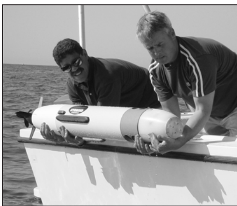
Photo 5: The first small commercial AUV, Remus, being launched by hand.
