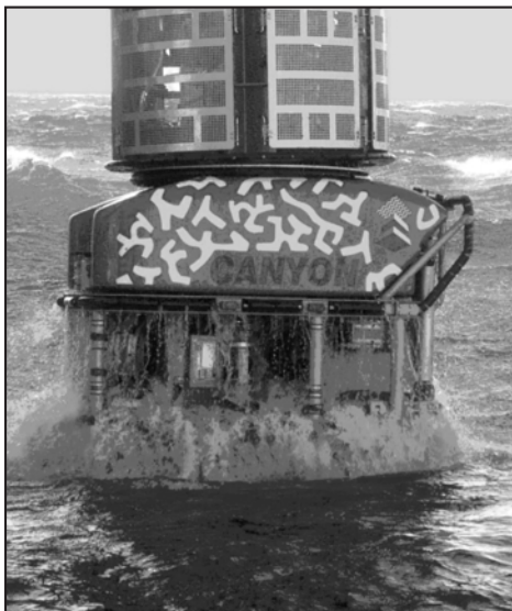
Photo 3: Canyon's Quest ROV being recovered off Hawaii in 2003 is an example of a workclass ROV.
