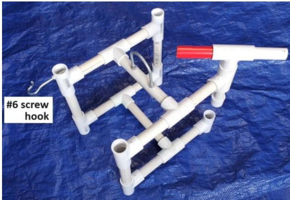
The irrigation system with the handle inserted through the 3/4-inch by 1/2-inch PVC tee.
