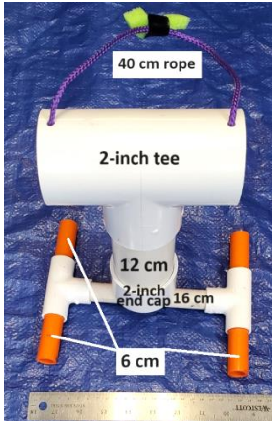
The Acoustic Doppler Current Profiler (ADCP) is constructed from 2-inch PVC pipe with a ½-inch PVC base. A 40 cm length of rope acts as the carrying mechanism for the ADCP.
