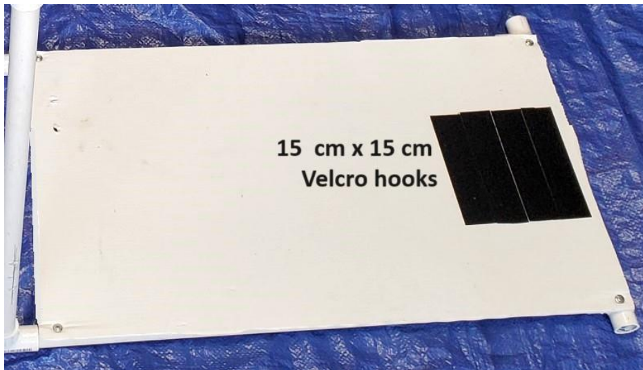
The transplant location for the brain coral is a 15 cm x 15 cm square of Velcro hooks.
