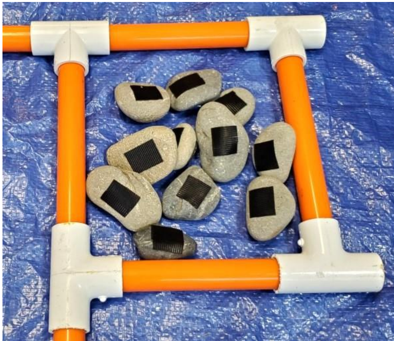
The sediment sample consists of Mexican Beach Pebbles with Velcro hooks attached.
