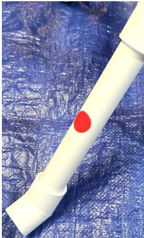
Corrosion is simulated by a red Velcro hook 1-inch circle on one of the “legs” of the subsurface structure.
