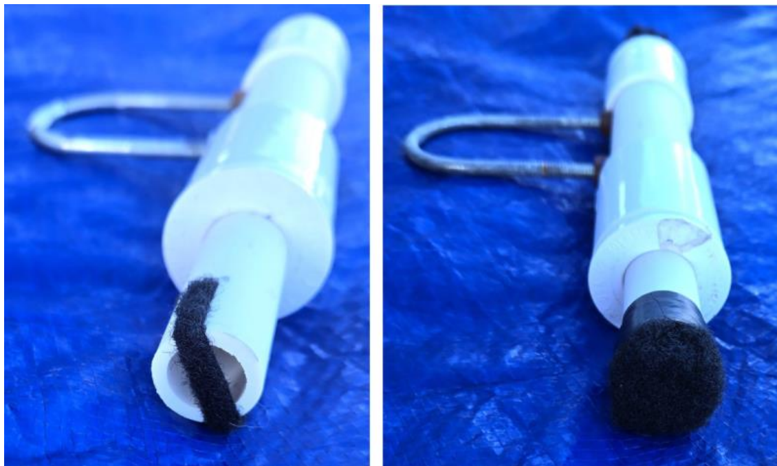
Left: The damaged thermistor has a thin 3 mm strip of Velcro loops on each end. Right: Each end of the new thermistor is completely covered with Velcro loops.
