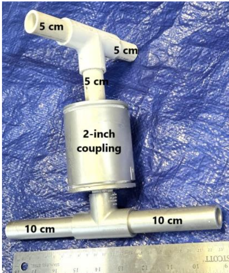
Both the old and the new sacrificial anode are constructed from 2-inch and ½-inch PVC pipe.
