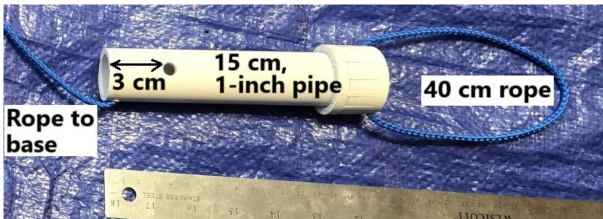
The hydrophone is constructed from 2-inch PVC pipe. A 40 cm length of rope acts as a carrying mechanism for the hydrophone. Flotation inside the 1-inch pipe makes the hydrophone section positively buoyant when the pin is pulled.
