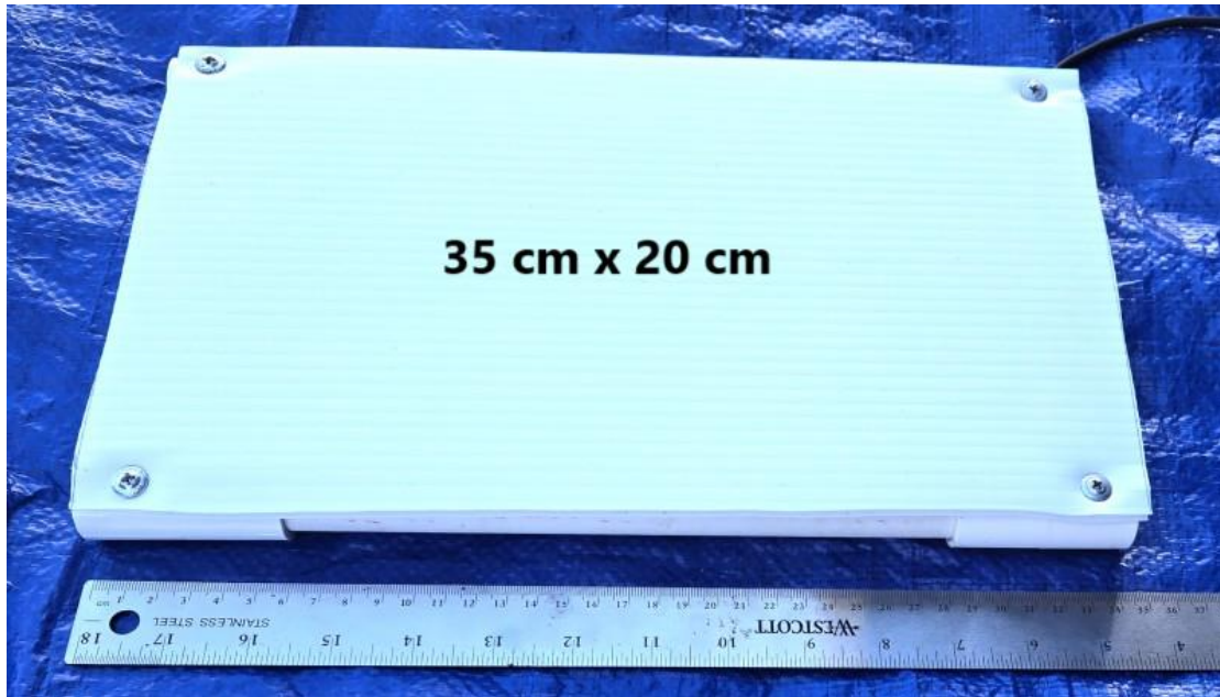
A 35 cm x 20 cm sheet of corrugated plastic tops the connector platform.
