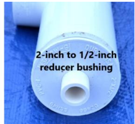
The connection port is constructed from 2-inch PVC pipe. Left: Top view. Right: Side view with a 2-inch to \frac{1}{2} -inch reducer bushing. \frac{1}{2} -inch pipe connects the port to the floating wind farm bottom structures.
