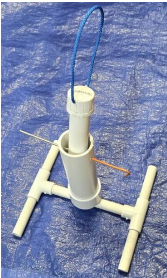
Left: The pin inserted, holding the hydrophone into the base. Right: The pin pulled, releasing the hydrophone to float, connected by a 40 cm length of rope, above the base.
