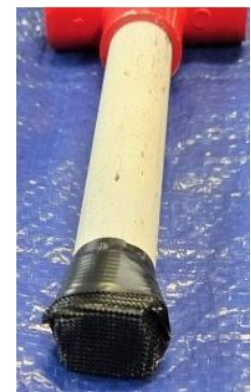
Left: The power connector is constructed from ½-inch PVC pipe. A #6 screw hook can be used to carry the connector. A 4-meter length of wire connects the power connector to the array's sub-surface structure. Right: A 6 cm x 4 cm rectangle of Velcro hooks covers the open end of the 15 cm length of pipe.
