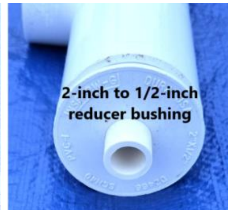
The connection port is constructed from 2-inch PVC pipe. Left: Top view. Right: Side view with a 2-inch to 1/2-inch reducer bushing. 1/2-inch pipe connects the port to the floating wind farm bottom structures.
