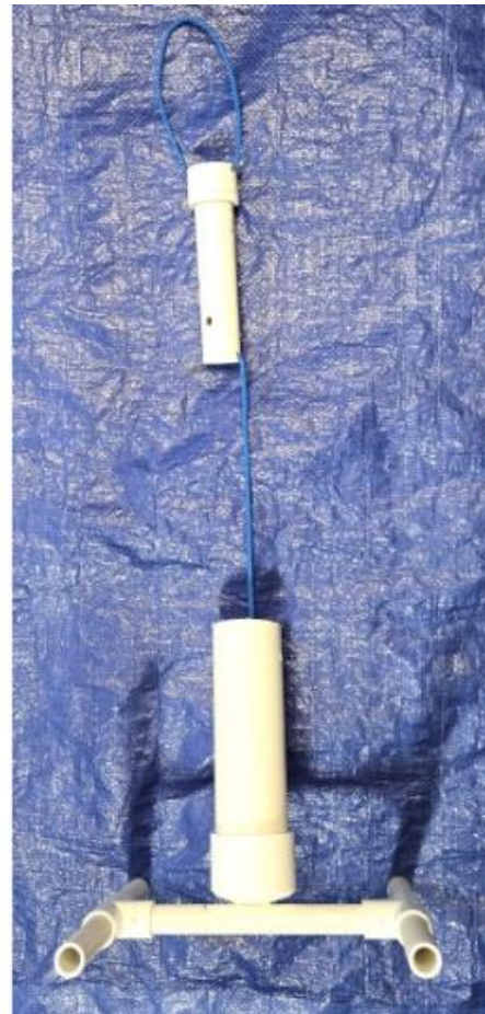
Left: The pin inserted, holding the hydrophone into the base. Right: The pin pulled, releasing the hydrophone to float, connected by a 40 cm length of rope, above the base.
