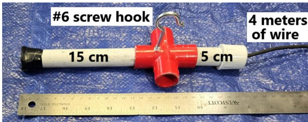
Left: The power connector is constructed from ½-inch PVC pipe. A #6 screw hook can be used to carry the connector. A 4-meter length of wire connects the power connector to the array's sub-surface structure. Right: A 6 cm x 4 cm rectangle of Velcro hooks covers the open end of the 15 cm length of pipe.
