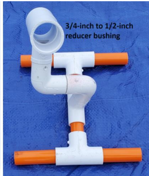
Left: Acoustic receiver front view constructed from 1/2-inch PVC pipe. Right: Acoustic receiver side view.
