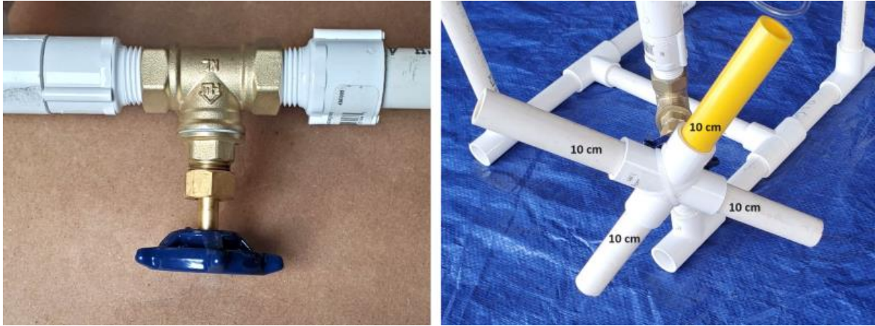
Left: The 1/2-inch brass stop valve has two 1/2-inch male adapters screwed into each side. A 1/2-inch gate valve can be substituted for the 1/2-inch stop valve if desired. Right: A 1/2-inch PVC cross is attached to the handle of the stop valve with a cable tie.
