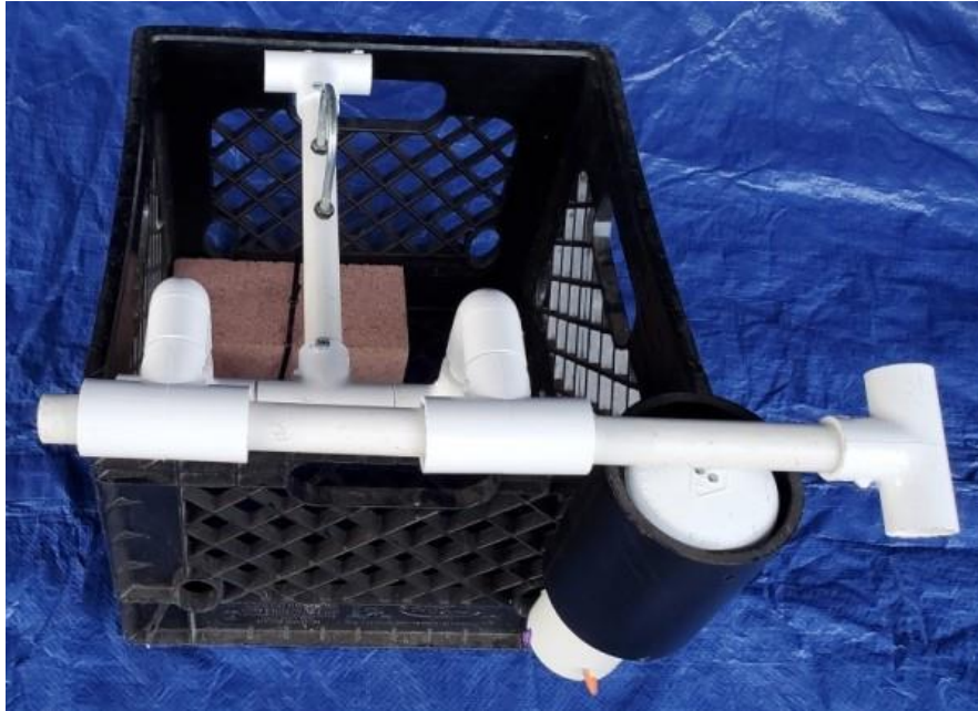
The multi-function node with the acoustic release pin holding the recovery float in place.
