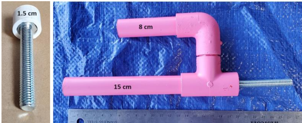
The branching coral is constructed out of \frac{1}{2} -inch PVC pipe. A 3/8-inch, 2 1/2-inch hex bolt is gently hammered into a 1.5 cm length of \frac{1}{2} -inch pipe.
