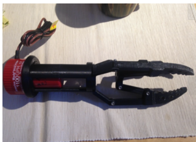
Fig. 7 Test design for an electric claw
