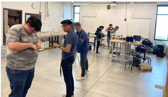
Fig. 13. Construction of the tether. Length: 15.24 m. Contents: pneumatic tubing, thruster connectors, and camera connections.
