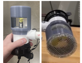
Fig. 15. Left: Final design of the thruster shroud. Right: Final shroud design with mesh on the top and sides of the shrouds.
