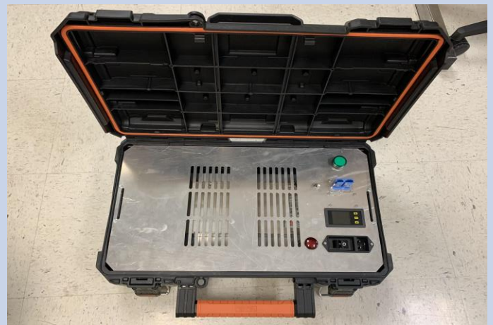
Figure 10: Talon's 48-volt power supply
