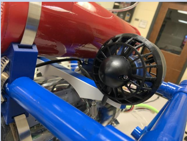
Figure 8: One of Talon's T200 thrusters, mounted parallel to the frame
