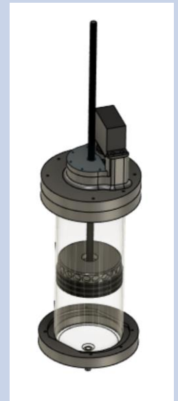
Figure 14: CAD rendering of GO-BGC float
