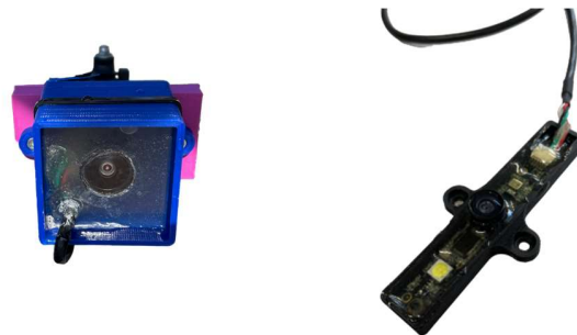
Figure 10: different waterproofing designs for the cameras
