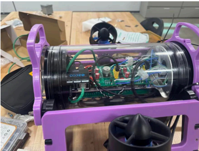
Fig 9. Enclosure of electrics after completion of ROV with no features
