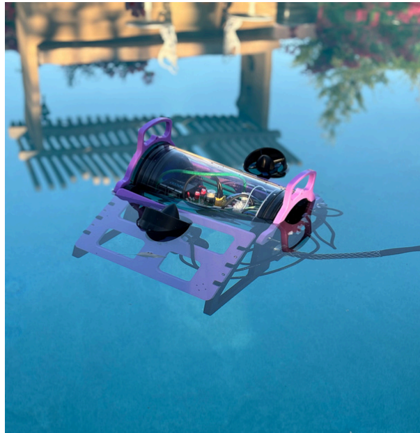
Fig 11. Nomad's positive buoyancy in first pool test
