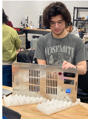
Fig 2. Electrical team member building 48-volt power supply.
