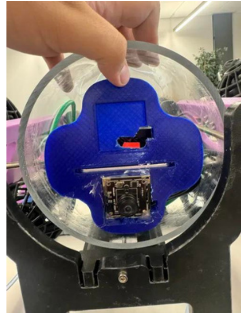
Fig 12. mounting piece designed by MATE for Nomad's Camera
