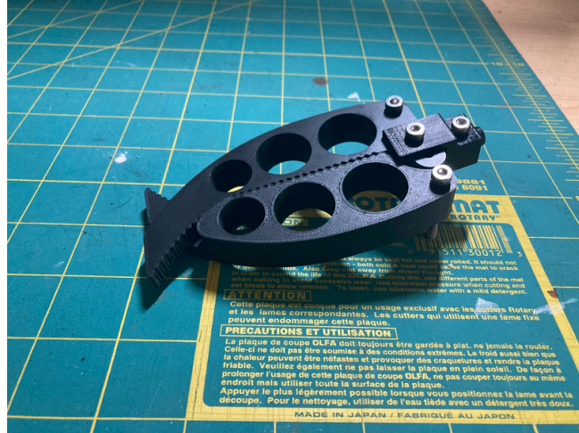
Fig 17. Renewed claw that can closed completely
