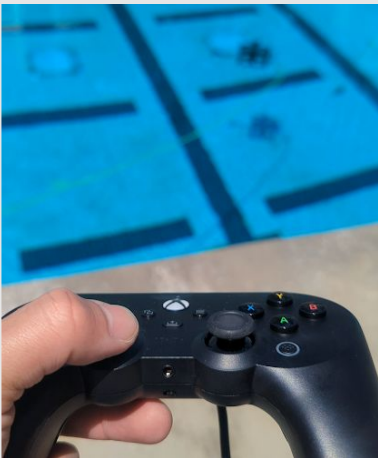
Fig. 18 Controlling the ROV with an Xbox Controller using the analog joystick
