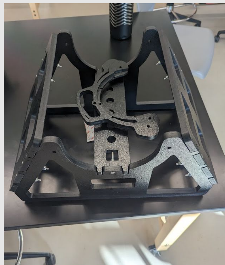
Fig. 13 HDPE frame assembled
