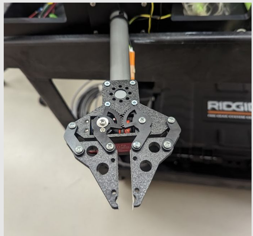
Fig. 27 Mechanical claw with 5V servo motor
