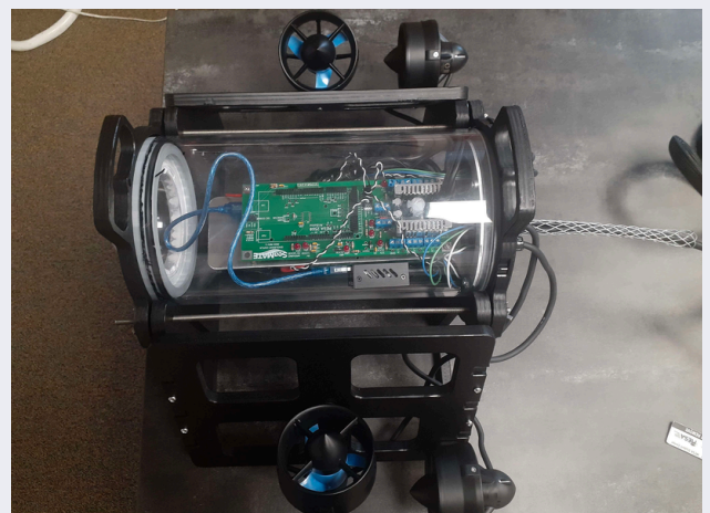
Figure 8: Thruster Placement on ROV
