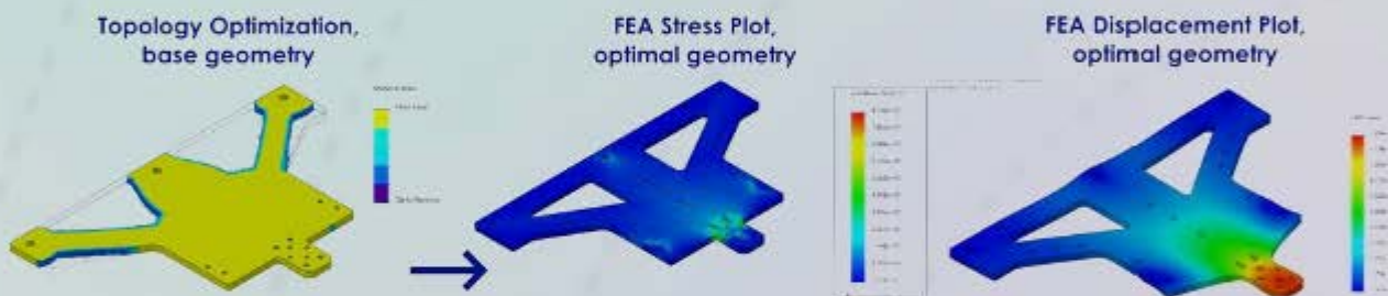
Figure 10: Topology optimization and static FEA of optimal HDPE middle panel
