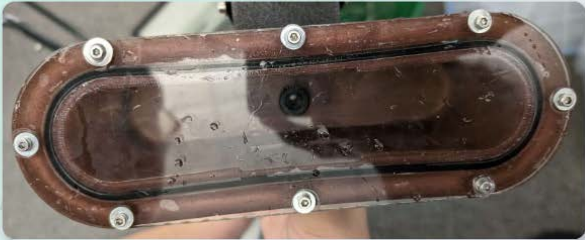
Figure 16: Deformed prototype of camera enclosure
